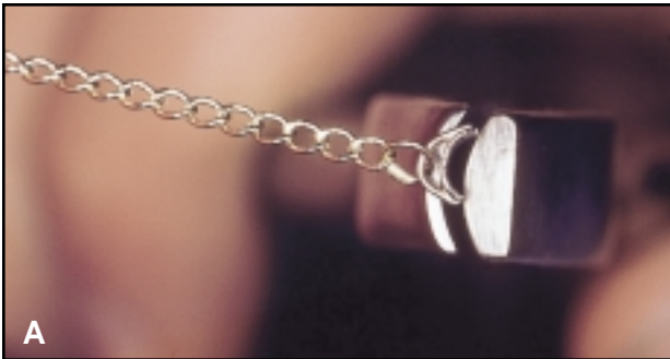
Fig. 2 A. U-Flex base opened with plier to reduce curvature. B. Base on left flexed open from original shape on right.
